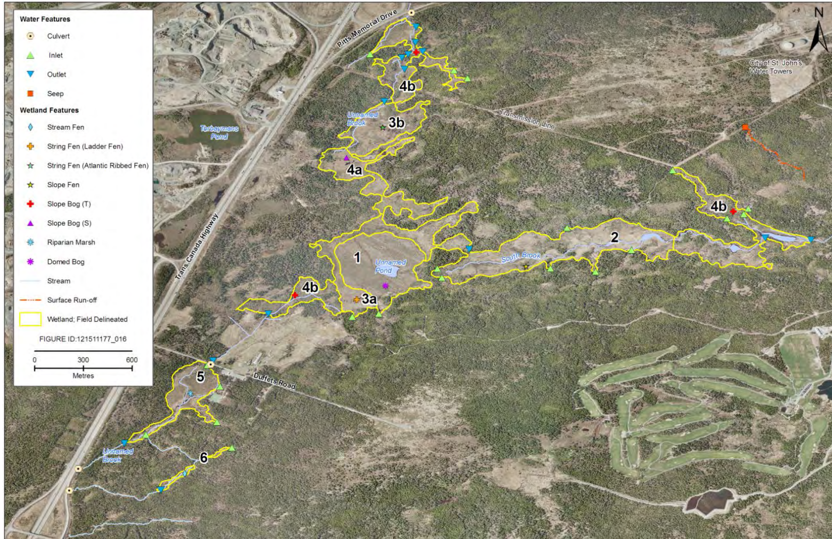
Figure 5-1 Assessed Wetlands Located on the Glencrest Property
